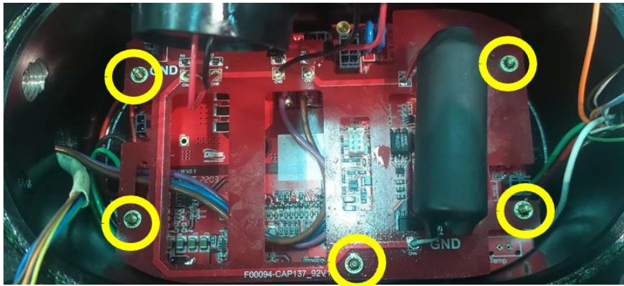
Figure 11 - Control Board Installation-8
