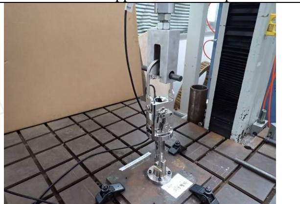
Photo "D" Tension Test - After testing
