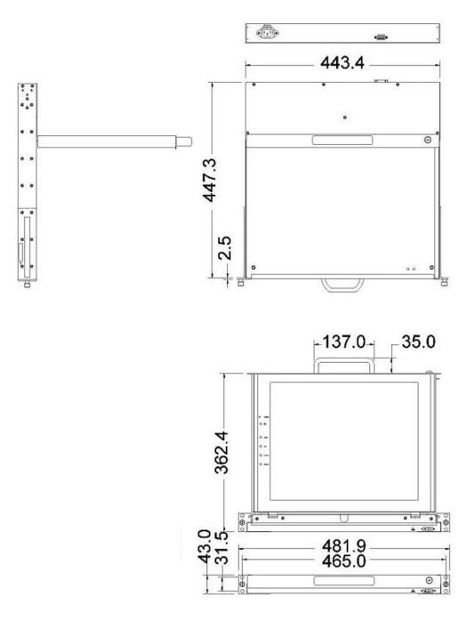
Figure 22 - 1U-LCD Monitor dimensions
