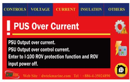
Figure 70 - Over current of power supply
