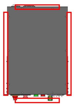
Figure 84 - Location diagram of the cross recessed pan head screws on the upper cover plate
