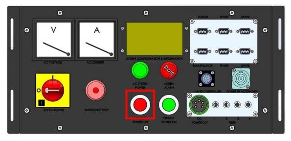
Figure 57 - Power off button diagram
