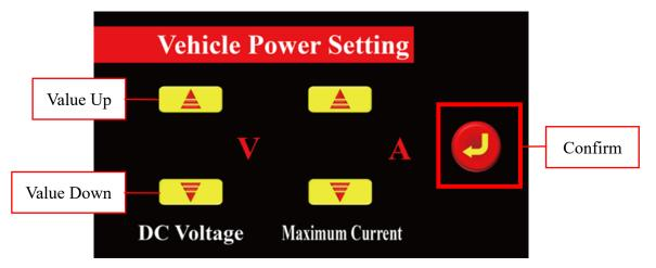
Figure 51 - 5U- Main Console Settings Screen Function Introduction
