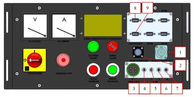
Figure 27 - 5U-Main console front panel pictorial diagram
