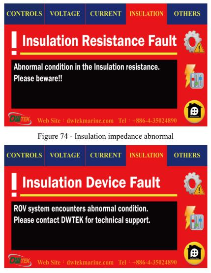
Figure 75 - Insulation monitoring device abnormal
