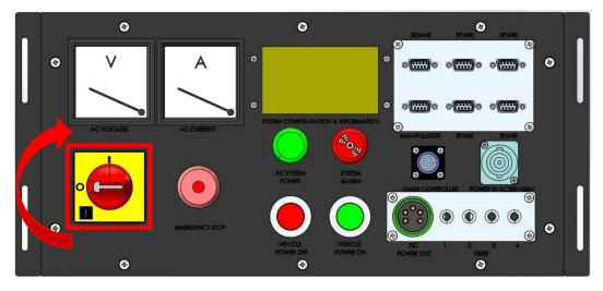
Figure 46 - System Start Knob pictorial diagram
