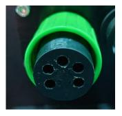
Figure 34 - VDC socket
