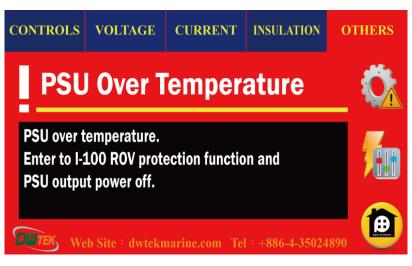
Figure 81 - Power supply temperature too high
