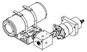
Figure 10 - Tilt Assy Unit Bevel Gear
