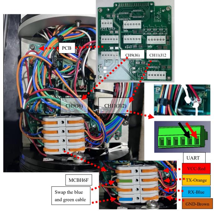
Figure 107 - How to change configuration of MCC
