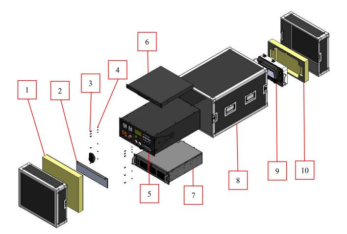
Figure 19 - ROV portable system exploded view drawing
