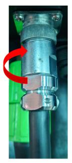
Figure 32 - Rotate clockwise to lock the signal connector in place
