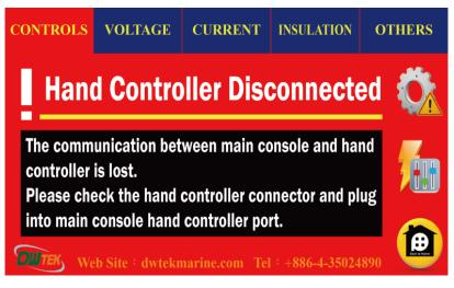
Figure 64 - Manual controller connection abnormal
