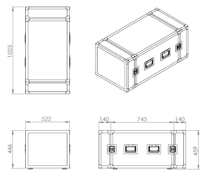
Figure 18 - ROV portable system dimensions
