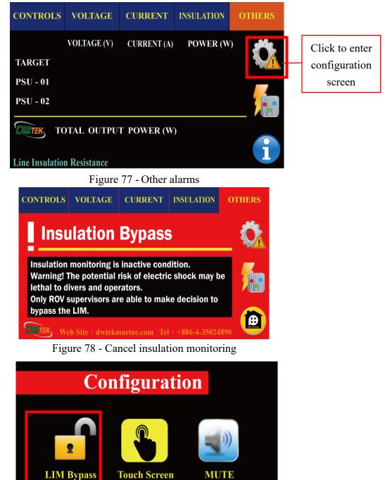
Figure 79 - Insulation monitoring not activated
