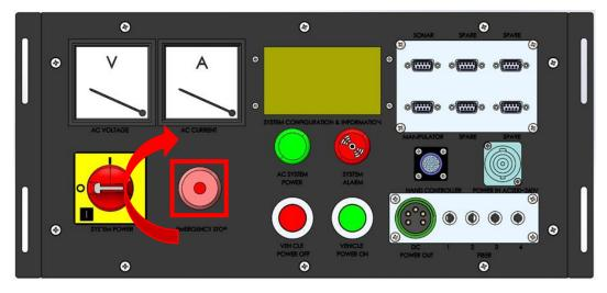
Figure 47 - Emergency stop switch release pictorial diagram
