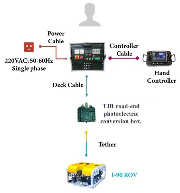
Figure 1 - I-90 ROV structure overview
