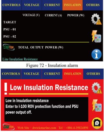
Figure 73 - Insulation impedance too low alarm
