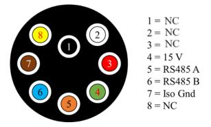
Figure 89 - Thruster connector pin assignment
