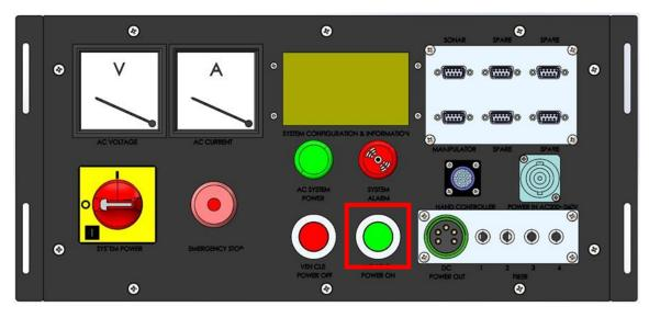
Figure 55 - Diagram of power-on button.
