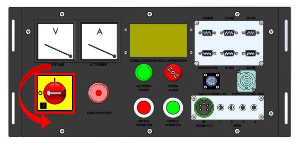
Figure 60 - Diagram of System Shutdown Knob
