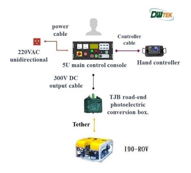
Figure 71 - Diagram of ROV connection to the 5U main control console
