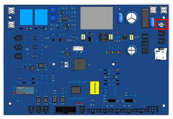
Figure 86 - Illustration of Spare Fuse Location
